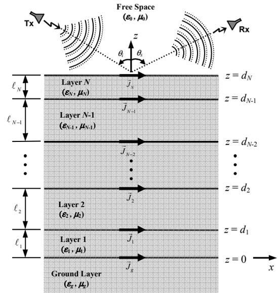
Figure 1. Geometry of the planar structure with  $N+2$  layers.
